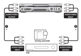
1 Connect a set of audio and video outputs on your VCR or camcorder to a set of inputs on this recorder.
